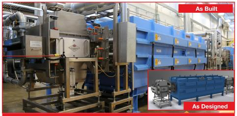
Carbon Fibre Low Temperature Furnace
